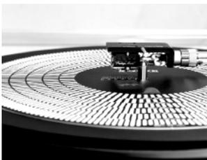
with stroboscopic disc and overhang gauge
